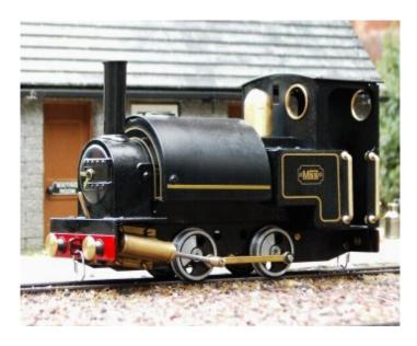
From my own experience of running the MSS locos, I have found that the Esbit fuel supplied with Wilesco's steam engines burns far better than the MSS fuel. All that is needed is a very small modification to the fuel tray.
