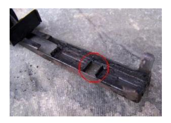
**Left -** The fuel tray as supplied has two tabs bent upwards in the centre to hold two halves of the MSS fuel in place.
