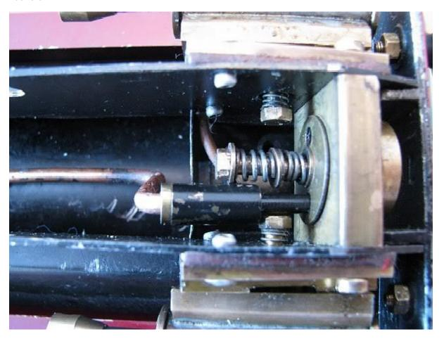
So some filing down of the T piece in these areas should ensure no interference with these pivot screws.
