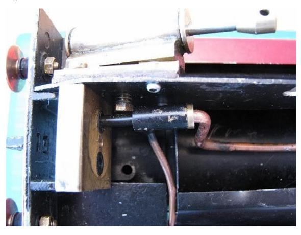
In this photo my regulator pivot screw has been modified with the addition of a 2nd spring & washers.
