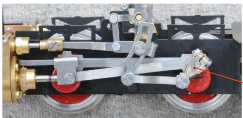
the return was correctly positioned it was held in place with Loctite (an adhesive-like fluid used to lock screws or nuts in place). Make sure that no Loctite comes into contact with the connecting and
