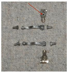
This shows the return crank and eccentric rod as shown on the Roundhouse picture and previous page. I did not drill for the pins but I did increase the clamping slot by making a very narrow cut for 1mm as shown by locating it into a vice and cutting it with a small saw. An M2 x 12mm socket cap and nut is supplied amongst the fixings provided by the Association as it is easier to clamp the return crank with a socket screw than with the cheese head screws. Once I had checked that
