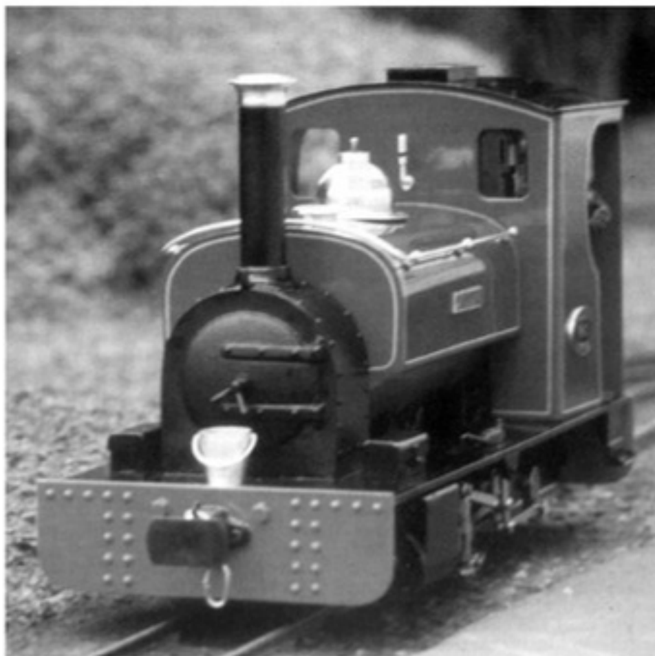
Left: A Merlin "Morris". Note rivetted buffer beam and smokebox. Compare with page 25.
